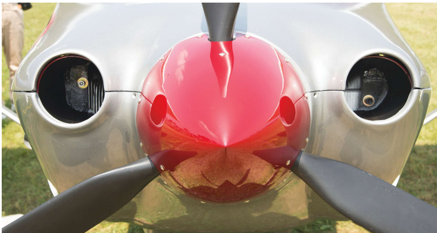
The hyper clean cowling not only contributes to overall performance but also cools the engine efficiently.
