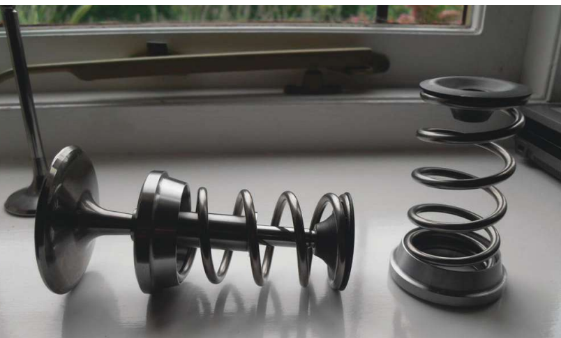
The ACE valve and its seat, keeper, and single valve spring unite to save weight, reduce stress, and transfer heat.
