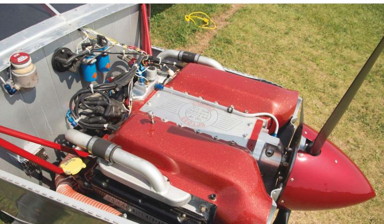
Close-fitting fiberglass plenums ensure that the Corvair's cylinders get maximum cooling.
