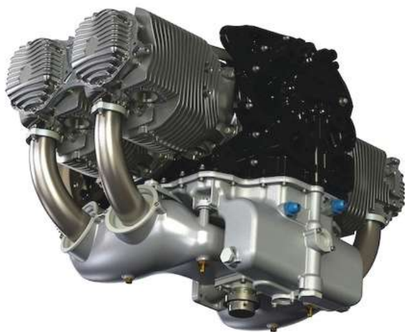
The AX50 GA 133 engine. The large intake plenum and oil sump are clearly visible in this view from below.
