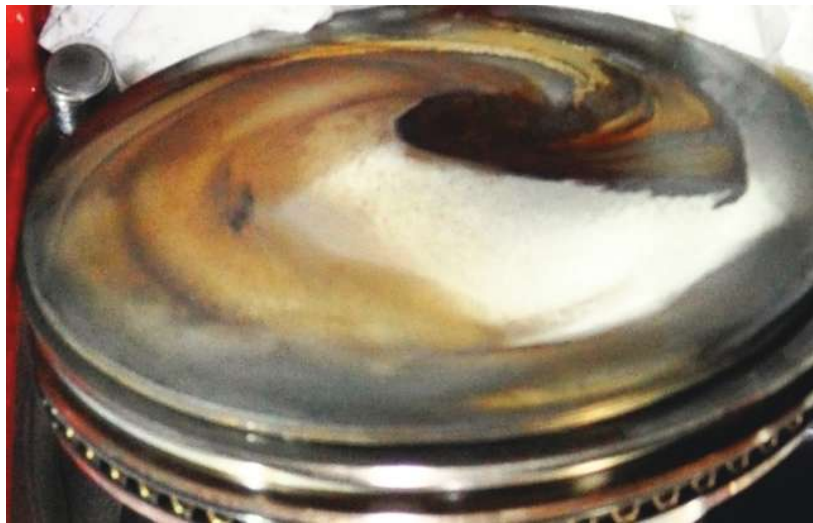
This photo of a piston from a test engine clearly shows the large amount of swirl in the ACE combustion chamber.
