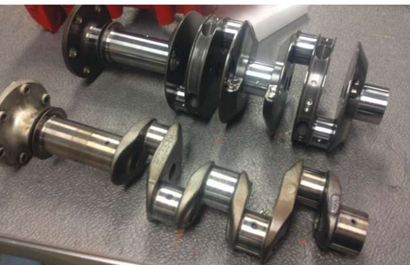
The differences in the original 360 crank and the AX50 crankshaft are obvious in this photo. Note that the ACE crankshaft is counterbalanced.
