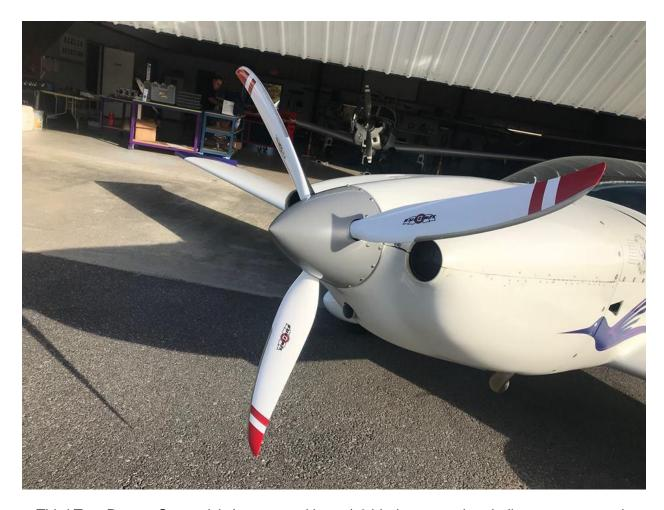
Third Test Prop: Sensenich (see a trend here..) 3 blade composite - hollow core - ground adjustable 58" prop.
