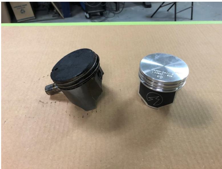
Removed piston (junk) and New Sealed Power Piston P/N L2206F .040
