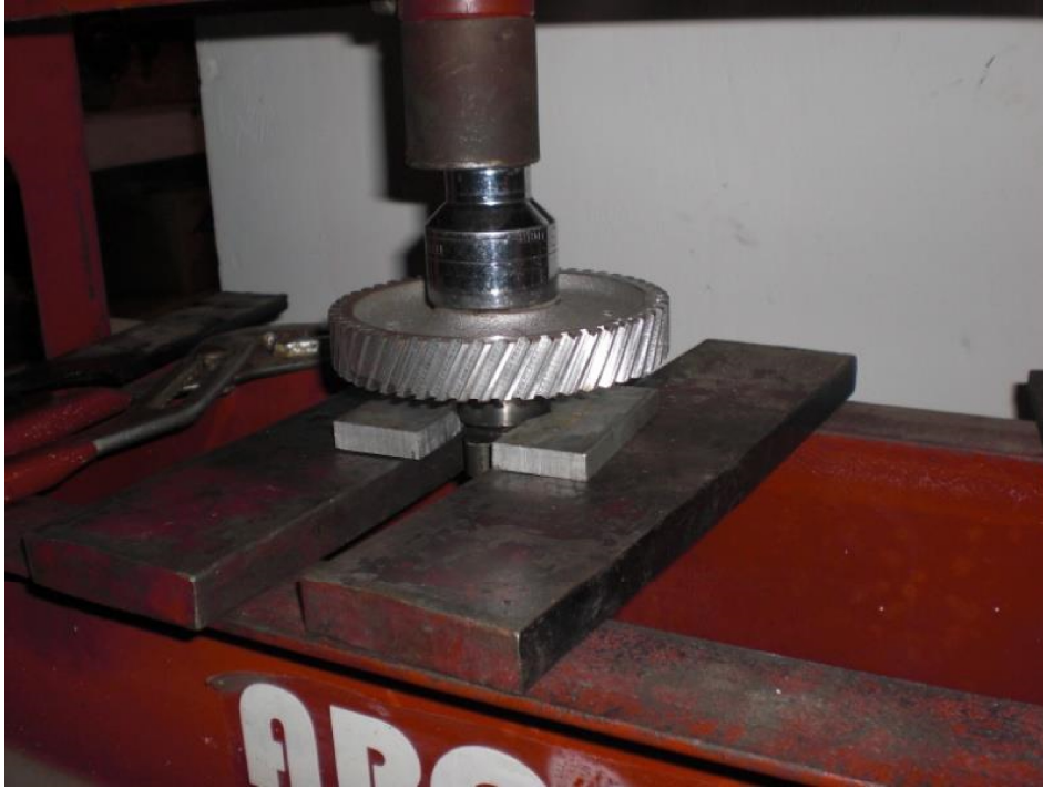
Camshaft gear pressed onto the camshaft in press.
