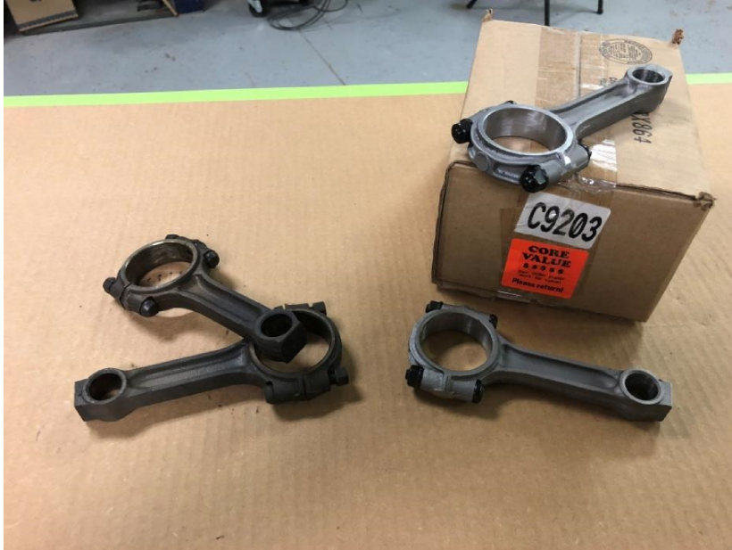
Rod cores and returned Reconditioned Rod set
