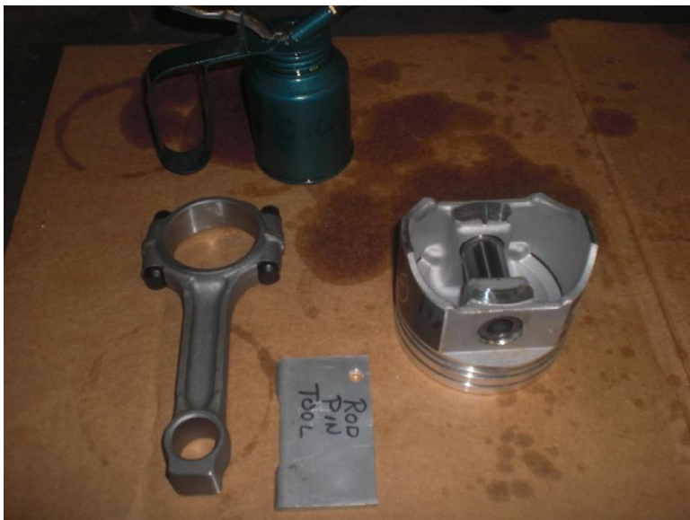
Reconditioned Rod and New TRW Piston before assembly.
