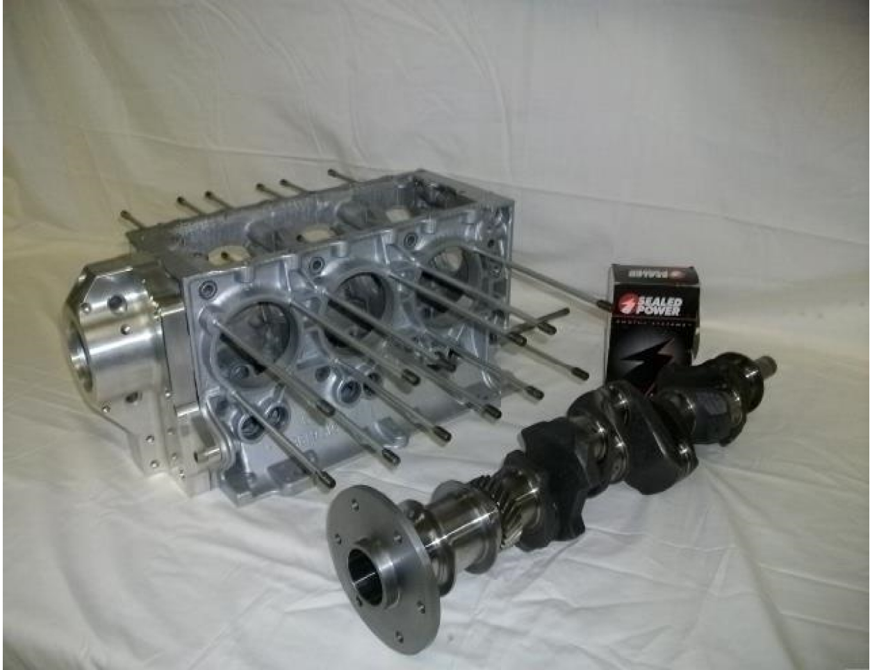
Finished Case halves with IFB Housing and Prepped Crankshaft.
