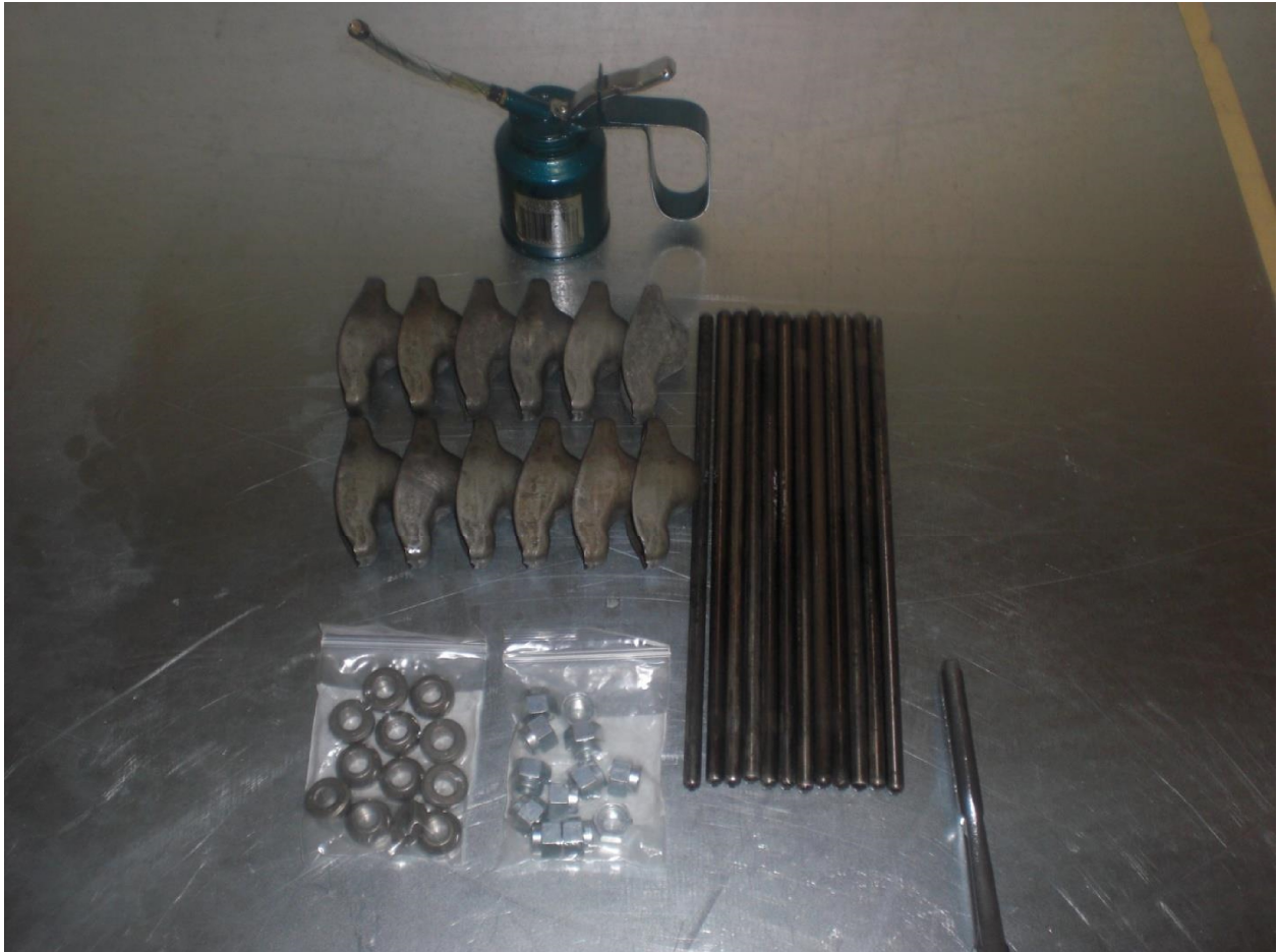
Cleaned pushrods and prepared rockers
