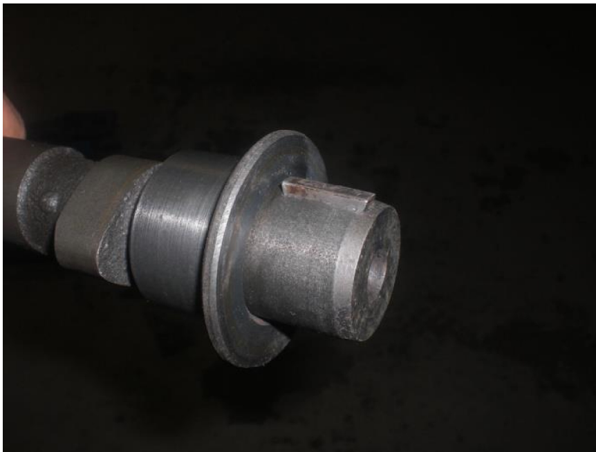
Thrust washer and Woodruff Key installed into camshaft.
