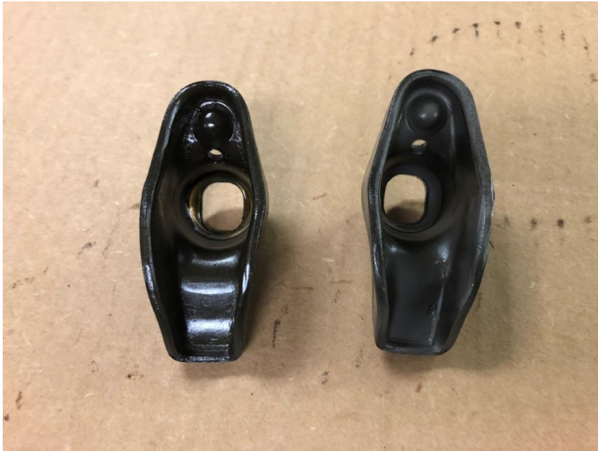
Removed rocker and prepped rocker
