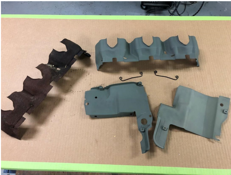
Before and after of Baffles...Rear tins primered
