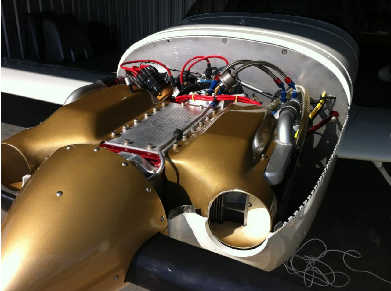
Spyder 120HP Installation in my Saberwing Prototype – pre-turbo
