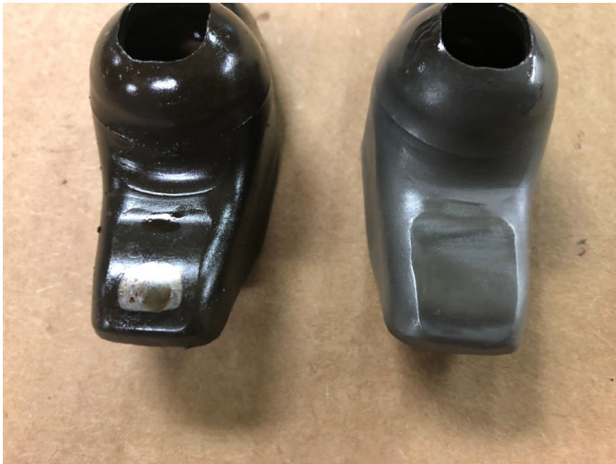
Note the stem contact surface area before and after prepping.
