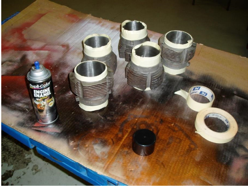
Prepping the Bored Cylinders for Paint.
