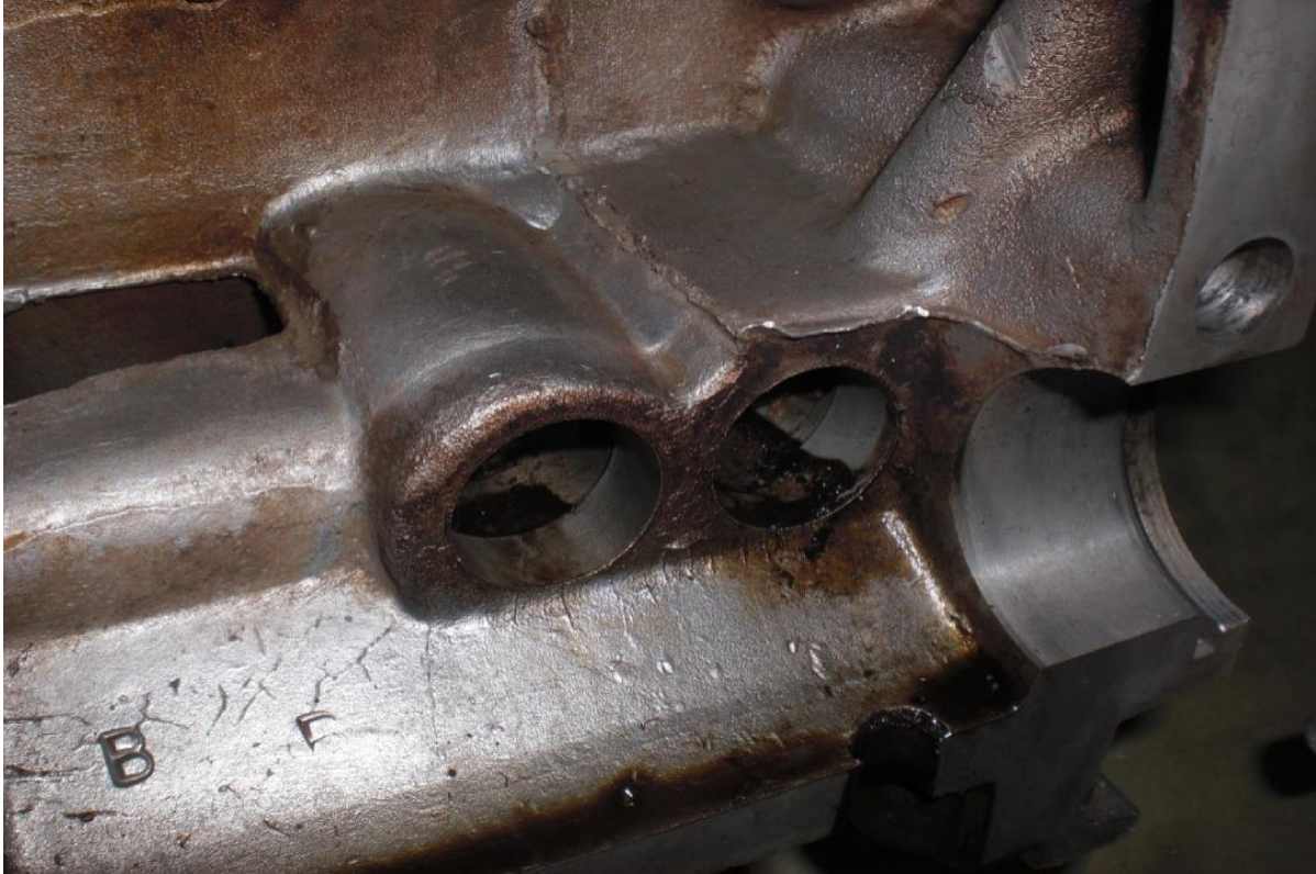
(Lifter bore area before cleaning and de-flashing)
