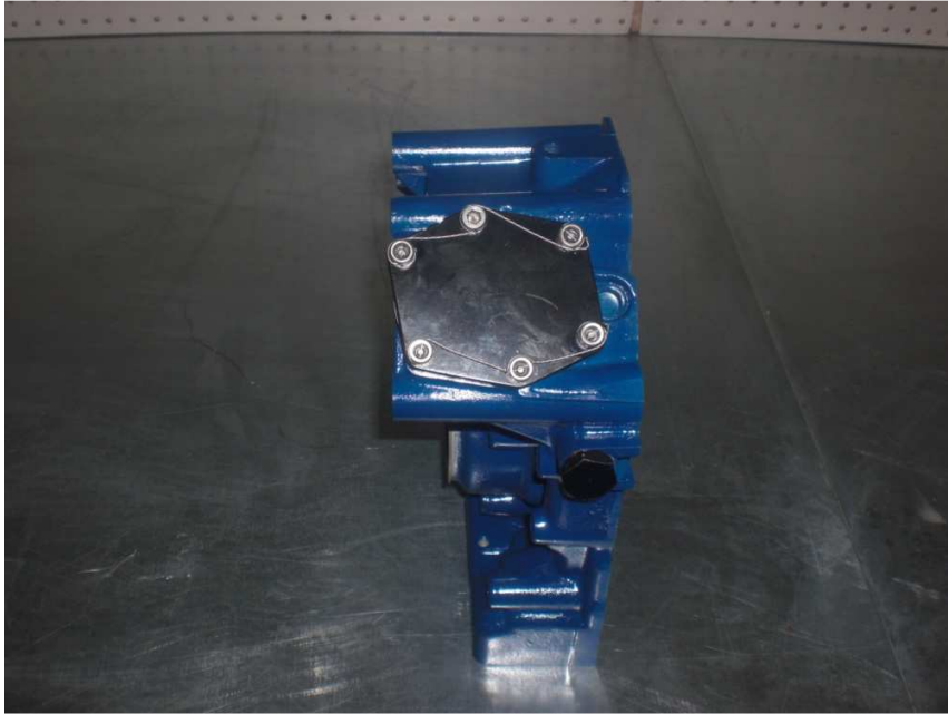
Fig 3. – Oil cover safetied and pressure relief valve installed
