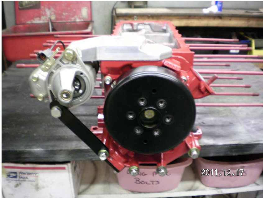
Fig. 4 – Lower Bracket bolted in place.
