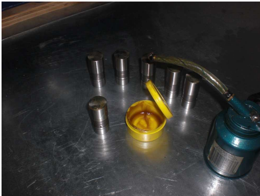
Fig. 2 – Cam lube on lifters – ready to oil
