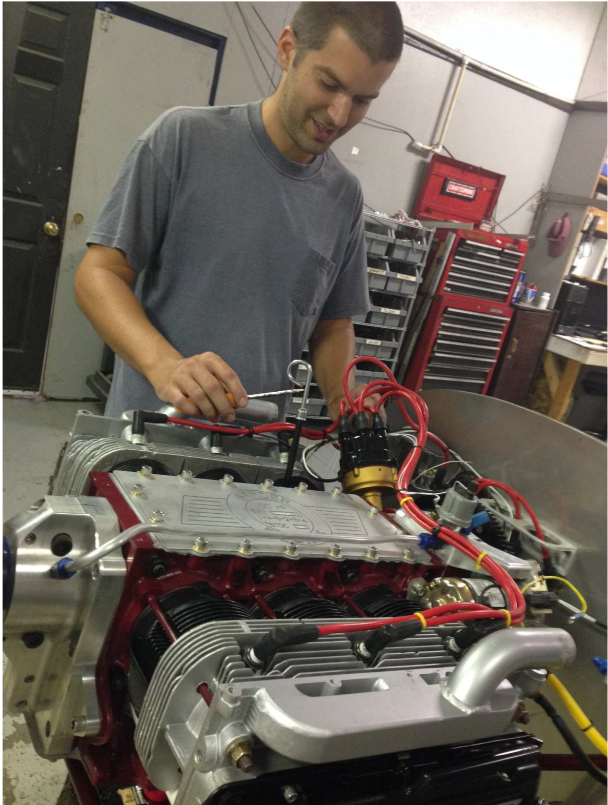
John finalizing his installation – a good view of the oil line and top cover.
