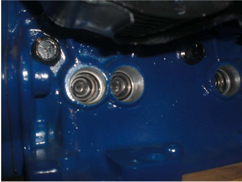
Fig. 3 – Lifters oiled and installed into bores
