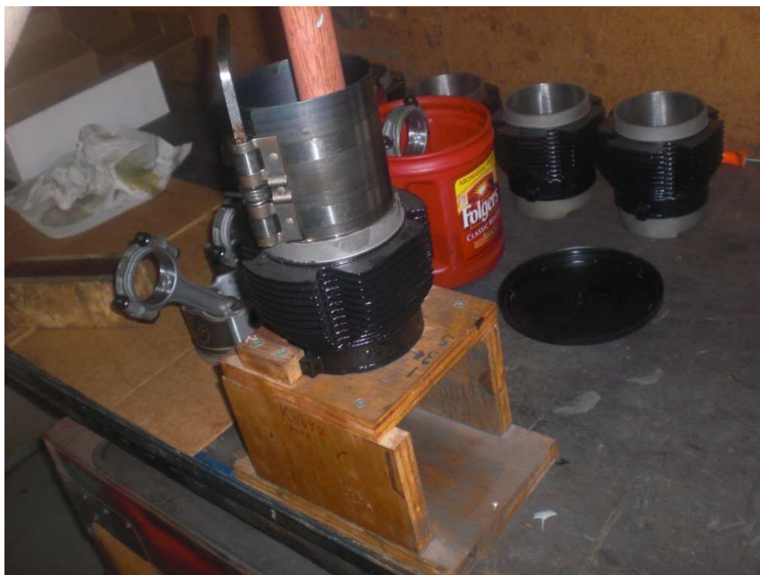
Fig. 5 – Remove the wooden block and firmly tap the piston into cylinder
