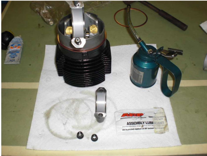
Fig 3. - Install rod bearing shell and copper base gasket on cylinder
