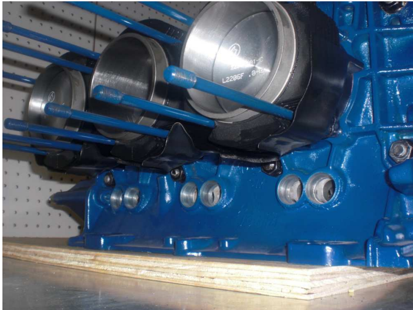
Fig. 8 – Installation of Baffle and clips (Notice the 3/4” assembly board under the case to provide clearance for the camshaft gear)
