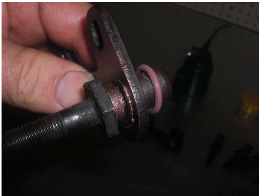
Fig. 6 – Rocker shaft installed on plate with o-ring
