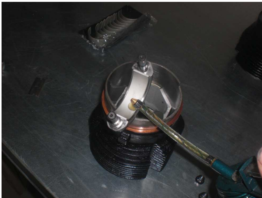
Fig 4. – Oiling bearing shell
