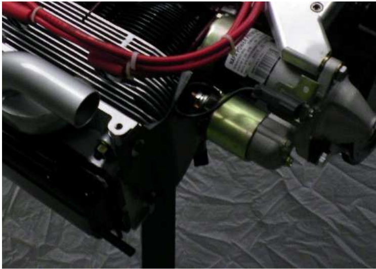
Tin (black) between starter and head/cylinder #2
