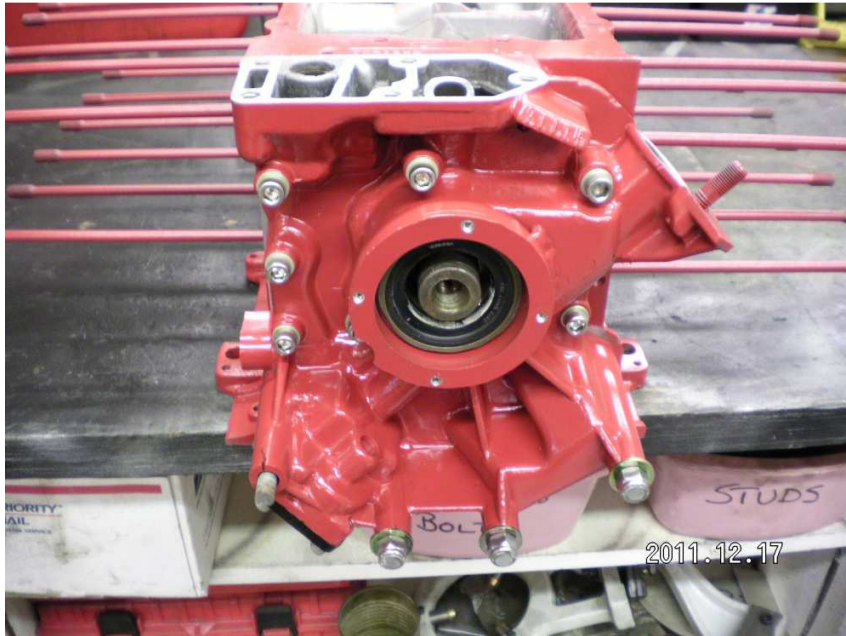
Fig 2. Rear housing installed onto case
