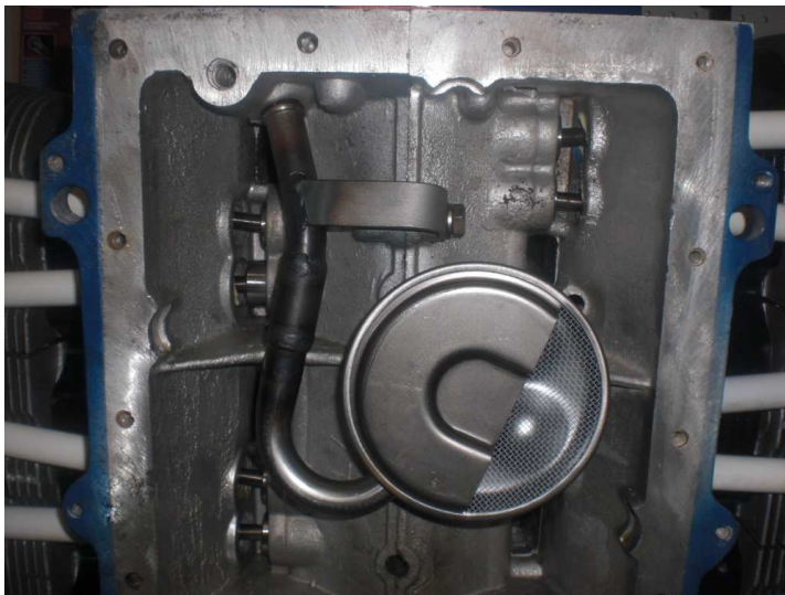
Fig. 3 – Typical oil pickup installation
