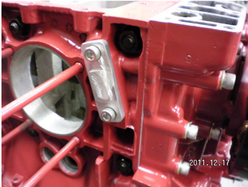
Fig. 2 – Block Off Plate Installed
