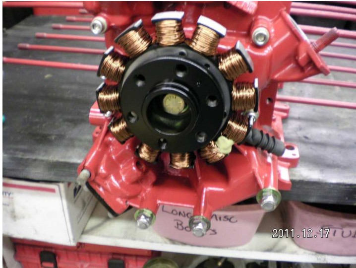
Fig 4 – Rear Puck installed and Torqued
