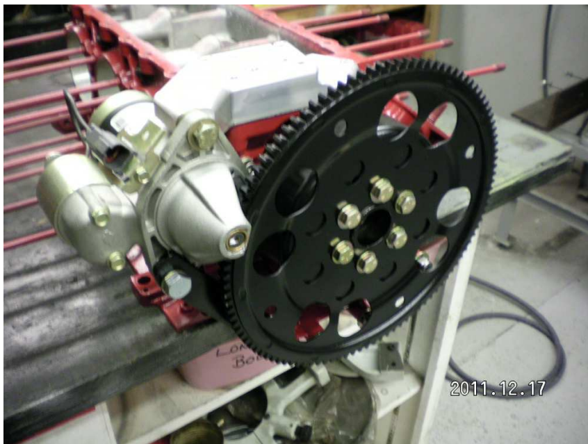
Fig. 5 – Starter and Ring Gear Finally Bolted
