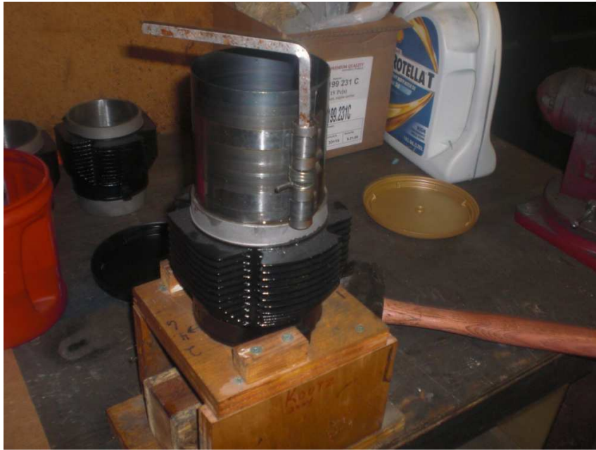
Fig. 4 - Install piston in correct orientation and compress rings
