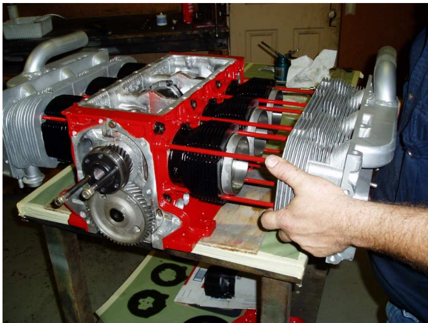
Fig. 9 - Installing head loosely to check for smooth rotation of parts. (note: no IFB in this installation picture)
