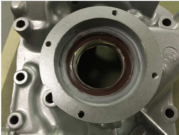
Fig. 5. - Rear Housing rear seal installed
