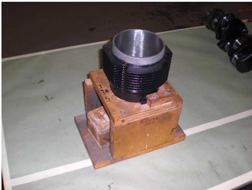
Fig. 3 – Cylinder in alignment Fixture - (make your own or call Azalea Aviation for rental/plans to build)
