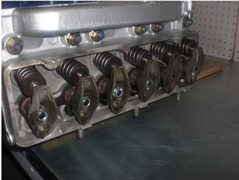
Fig. 3 – Rockers installed and ready for adjustment
