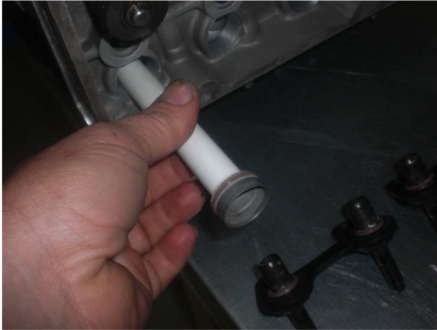
Fig. 7 – Installing pushrod tube
