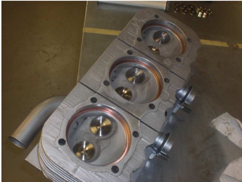
Fig. 5 – Cylinder Head with gaskets installed
