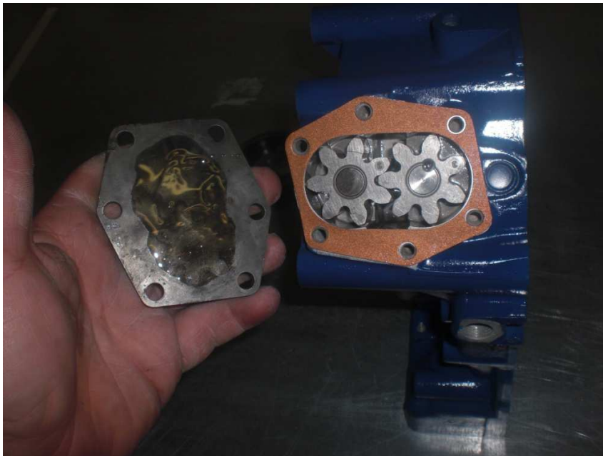
Fig 2. – Installing Cover plate
