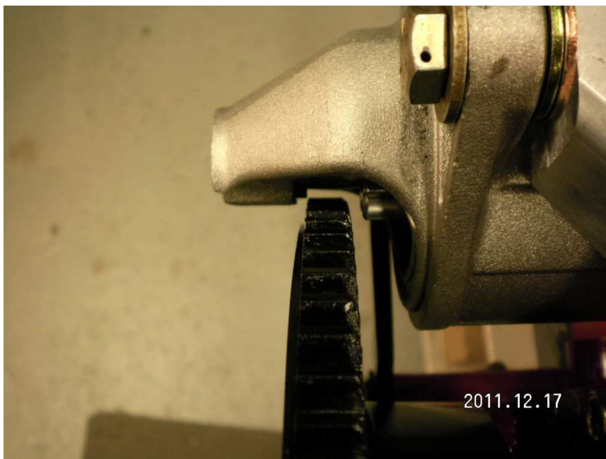
Fig. 3 – Ring gear to Bendix clearance
