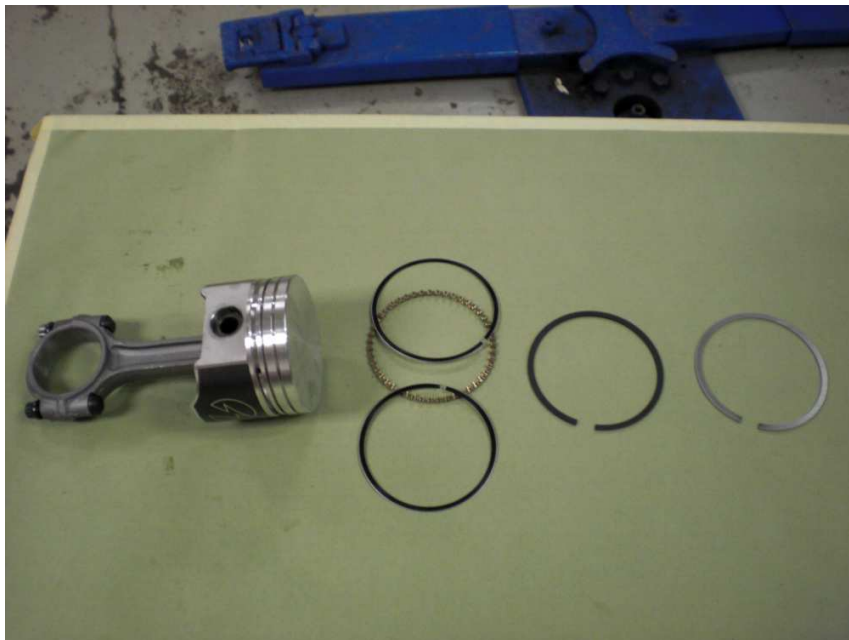
Fig. 1 – Rings ready for Installation
