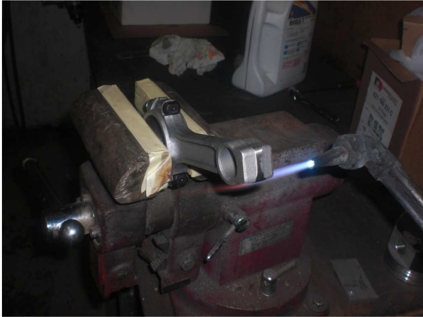
Fig. 3 – Heating up Rod small end (brownish color)
