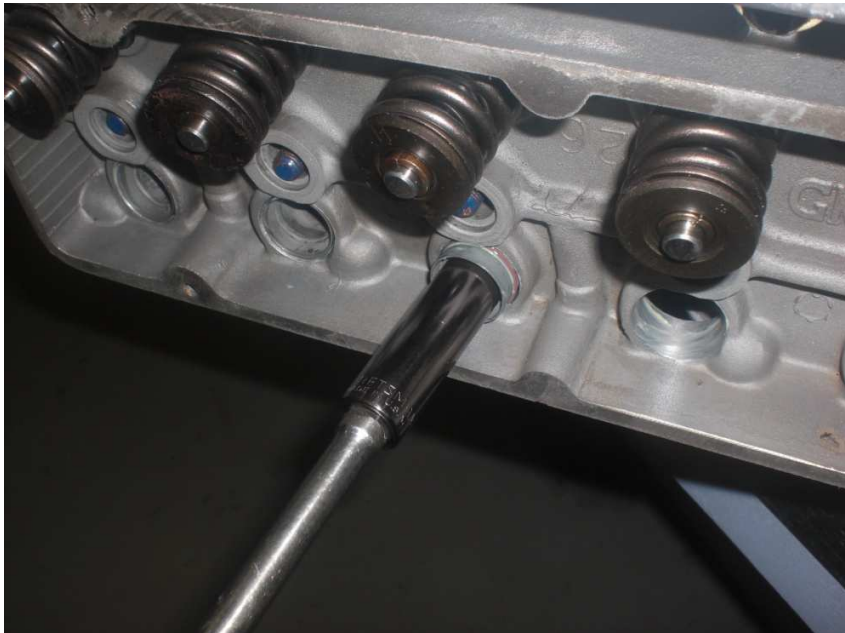
Fig. 8 – Pushing pushrods into position
