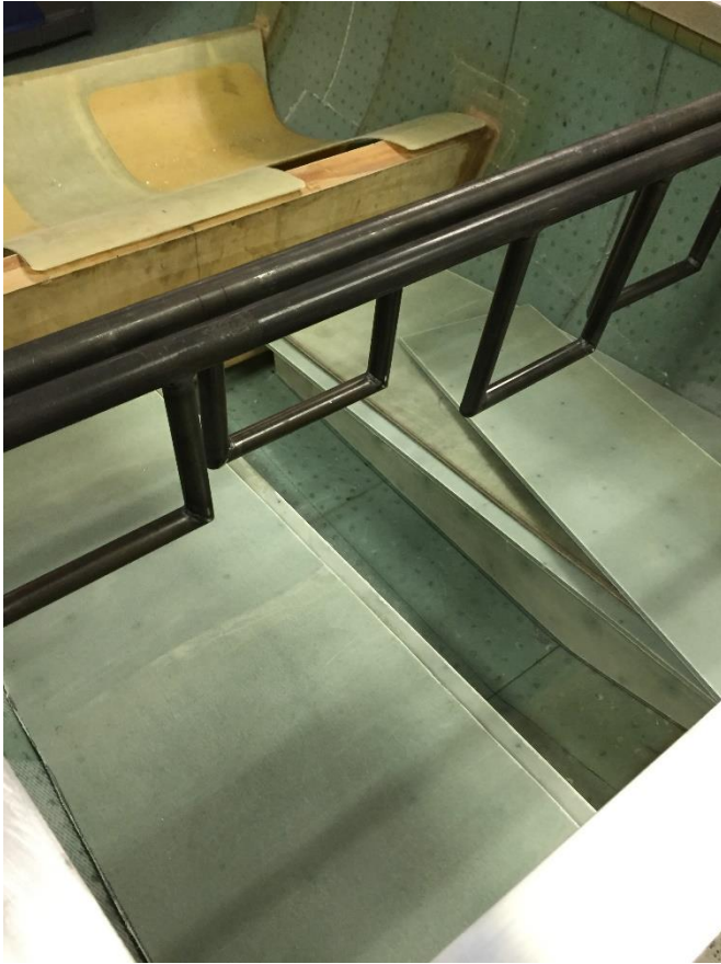
Hanging rudder pedals ...forward floors...
