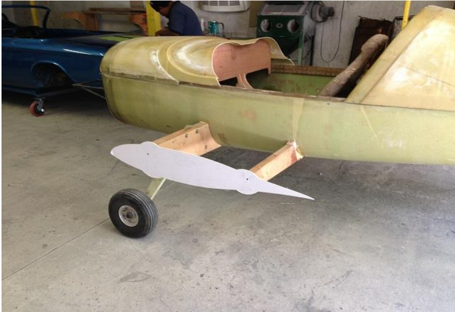
Gear installation and beginning stub wings
