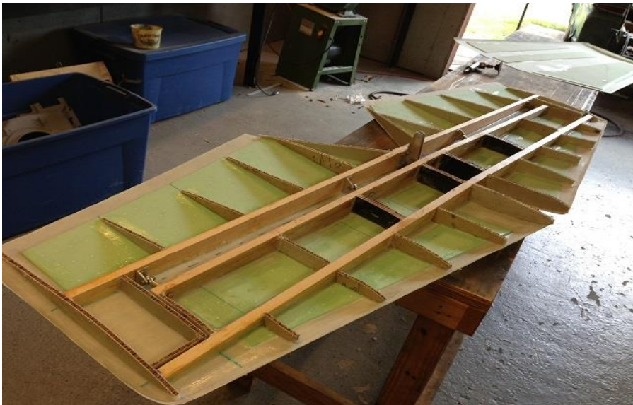
Horizontal/Elevator Assembly - skin in background
