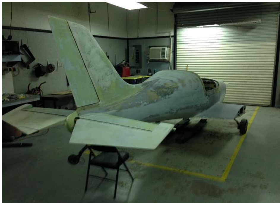
Final bodywork on Fuselage before primer
